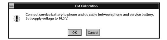
When external power is connected and user selects Yes to continue, the application displays the **Energy Management Calibration** dialog box:
